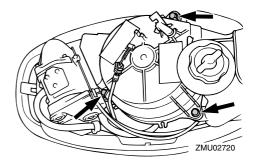
Reinstall two bolts to secure the fuel tank.
